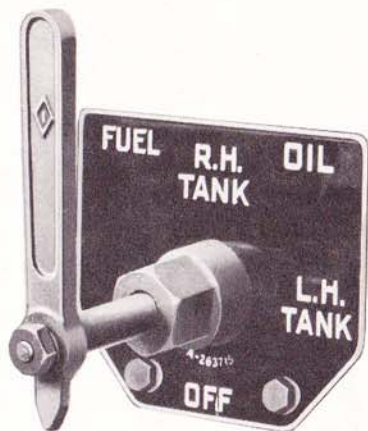
Figure 83—Fuel Tank Selector Valve
